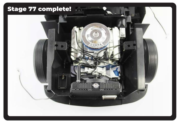
You will add the strut bar, battery, oil filter and pipes to the engine section.
